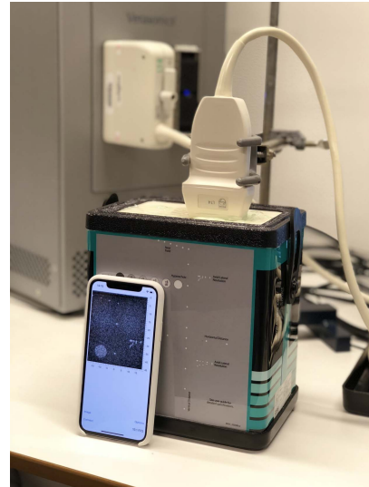
Fig. 1. Complete setup of the ultrasound probe imaging a phantom with the research scanner streaming the channel data wirelessly through the router before it is received, beamformed, and displayed on the iPhone. A demo video is available at https://youtu.be/oN8cwysGxyM .
