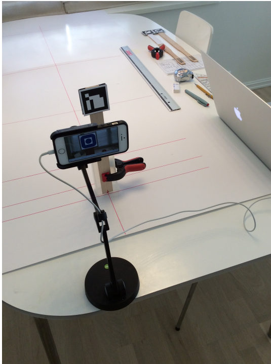
Fig. 6: Depth and rotational accuracy experimental setup.
